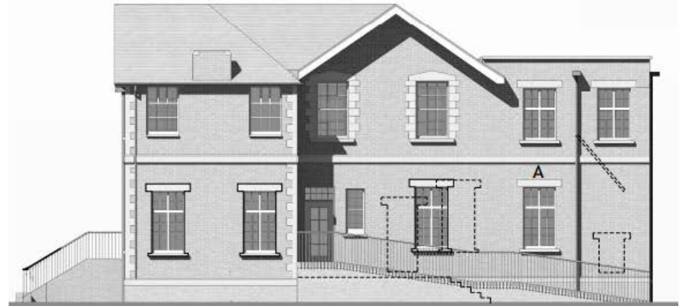
elevation to courtyard 2 new windows to match type A existing steps and porch removed and replaced with new ramp existing opening bricked up to match and dp repositioned existing window moved to line up with window above
